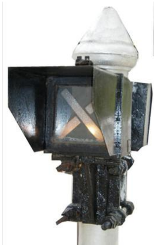
Fig: 7.6 (a) SHUNTING PERMITTED INDICATOR
