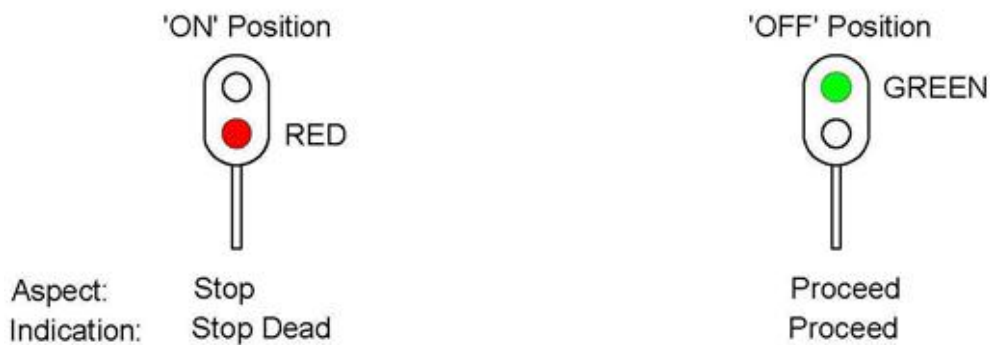
Fig.4.18 (a) Two aspect Colour Light Stop Signal
