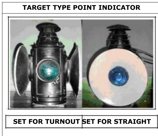
FIG. 7.14 (a) TARGET TYPE POINT INDICATORS
