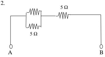
Calculate the total resistance across terminal A and B.
