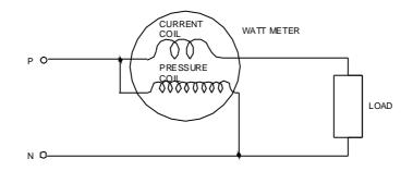
The circuit diagram for measuring the power of a single phase load with watt meter is shown above. The watt meter has got 4 terminals . Two terminals for current coil and two terminals for pressure coil. One CC terminal and one PC terminal is shorted and given phase supply. Other end CC terminal series to the load and PC terminal given neutral . Now the watt meter read the load power.
